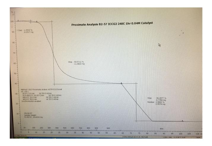
Appendix 1. Mass loss as function of temperature for sample of PCS biofuel produced from A/D digestate.
